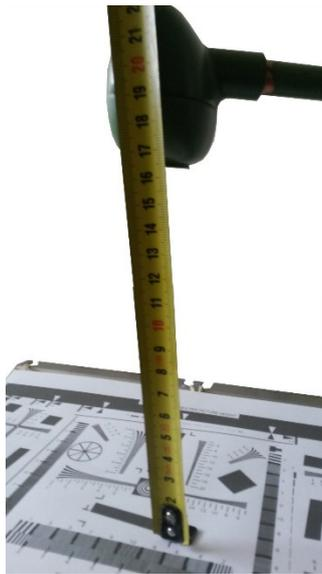
Figure 11: respect the ~17cm between the foil and the optic
