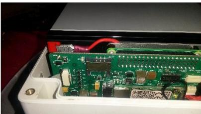
Figure 3: The SIM card slot
