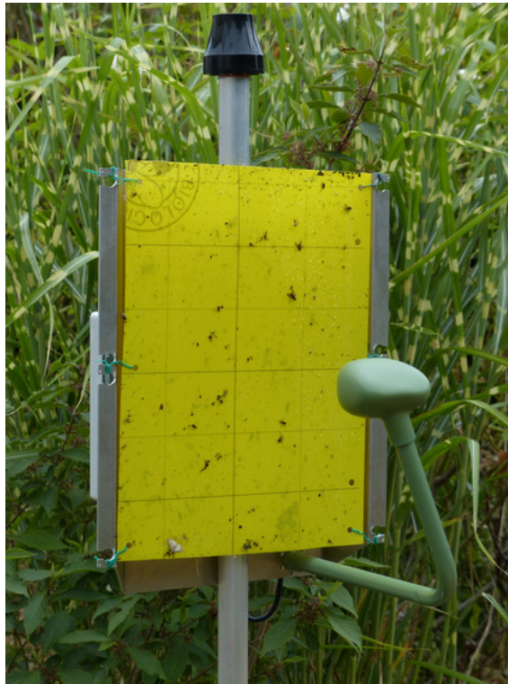
Figure 2: e-GLEEK® equipped with one A4 sticky sheet
