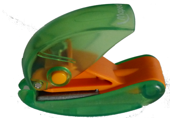
Figure 4: Small puncher used to make fixation holes in the glued sheet
