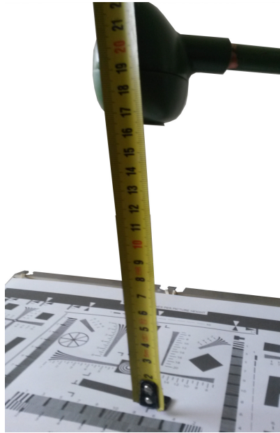
Figure 9: Distance between sheet and optic element
