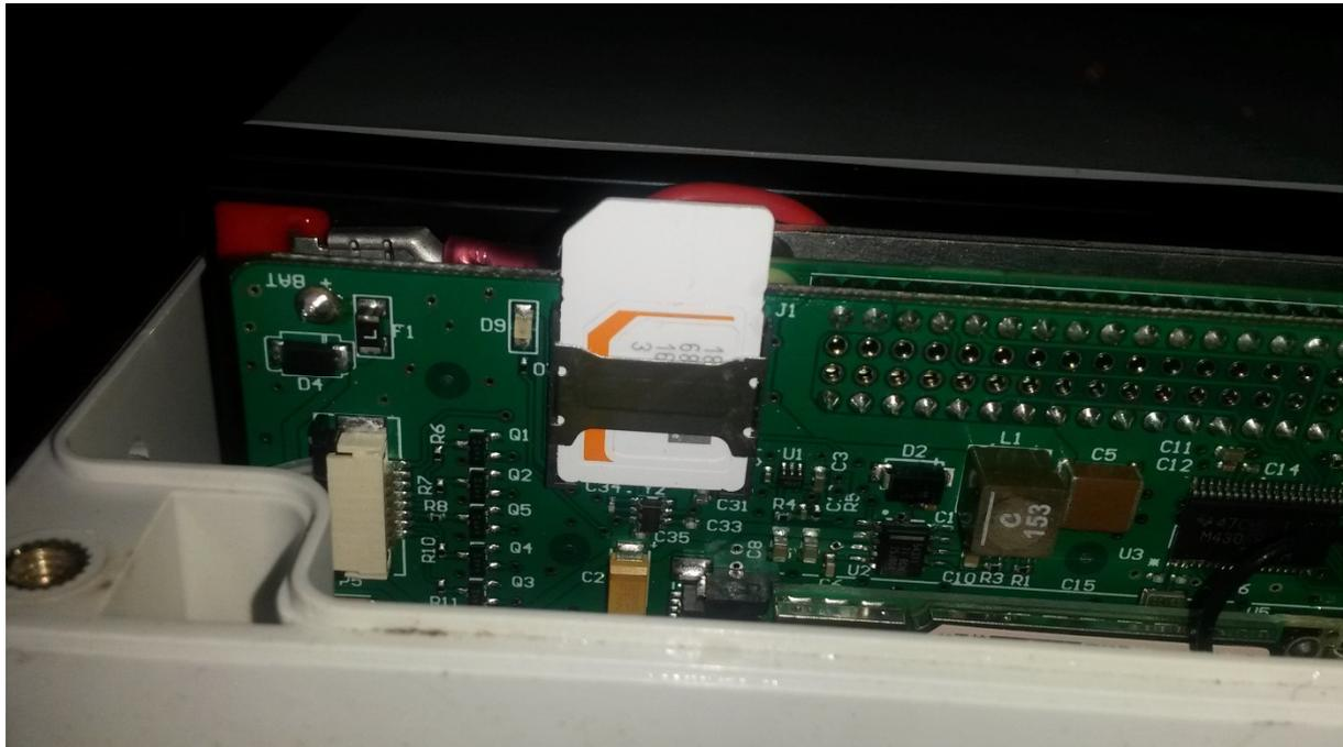
Figure 2: The SIM card correctly inserted in the slot
