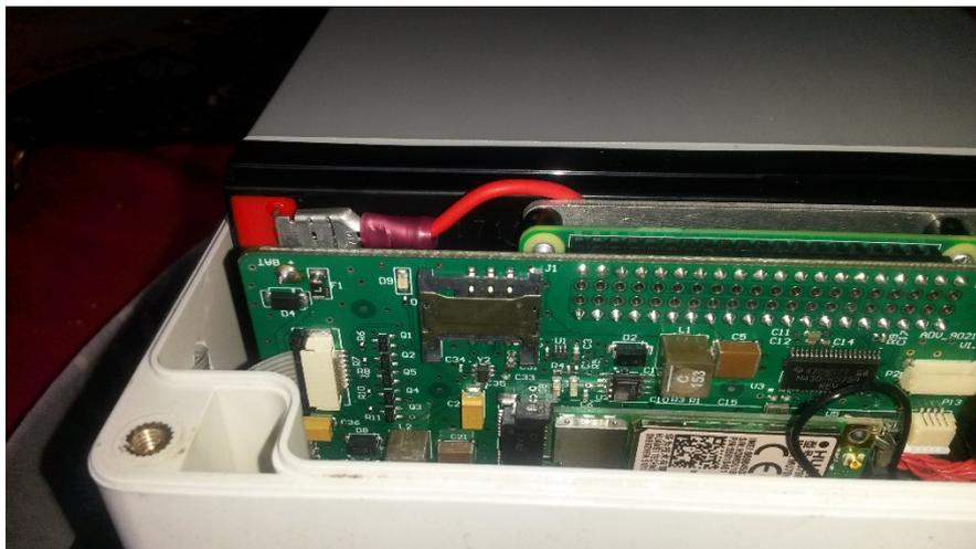
Figure 1:Slot for the SIM card
