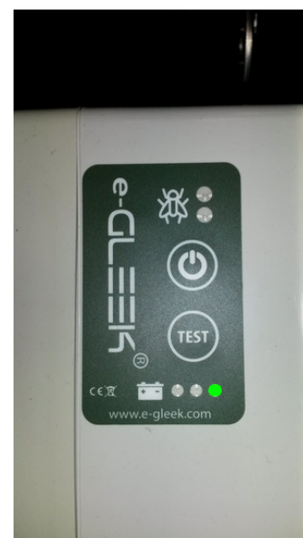
e) 2 consecutive pushes on the TEST button will initiate the Wifi hot spot (blinking diode battery) SSID: e-gleekxxxxxx Password: tgv44air!
