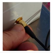
Insert the antenna cable through the hole Put the spacer and the nut. Thighten. Connect the cable to the golden connector at the top of the electronic white box
