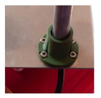
Insert the optic cable through the hole.
